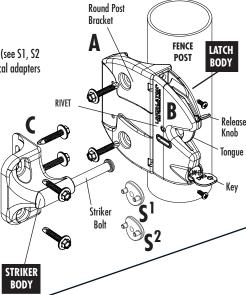
The External Access Kit (EAK) allows a gate to be opened and locked from the opposite side to the latch. Once the "handing" is determined, The EAK is connected to the Latch Body by a Push Rod.
