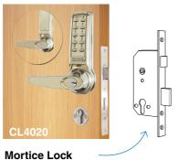
Euro profile mortice sash lock with deadbolt and latchbolt. With the deadbolt thrown it denies access to code users. Supplied with Euro profile cylinders and three keys.
