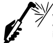
Warning: Hinges will be severely damaged if electrical welding current is not properly grounded and will result in the warranty being void.
